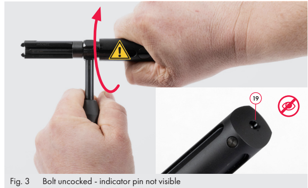
Fig. 3 Bolt uncocked - indicator pin not visible
