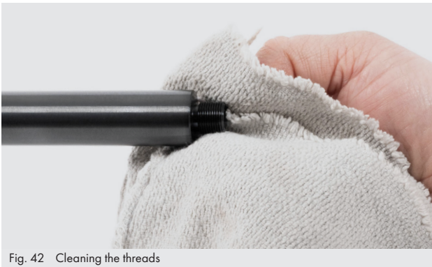
Fig. 42 Cleaning the threads
