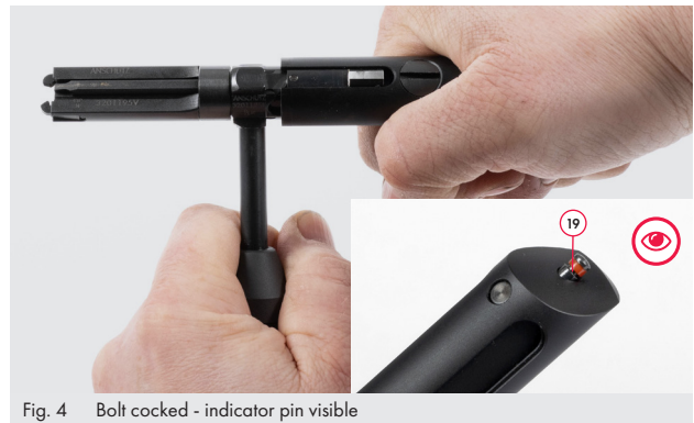
Fig. 4 Bolt cocked - indicator pin visible
